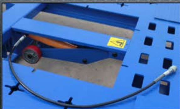
Tilt Deck w/ quick disconnect connection
