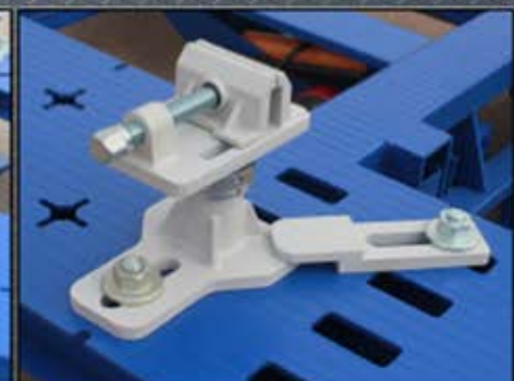
Adjustable height Pinch Weld Clamp Assemblies
